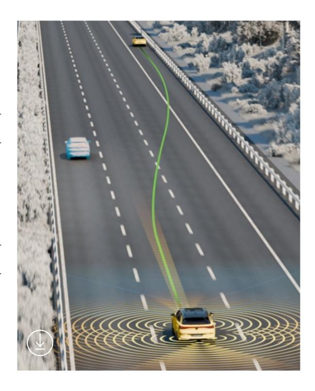
68 km/h. When Travel Assist is active, it predictively integrates upcoming traffic routing, such as corners, roundabouts and junctions, into vehicle control and the displays. For instance, if there is a corner ahead and the set speed is too high for taking the corner, the system shows the message 'Corner ahead' and the speed is adjusted accordingly<sup>2</sup>. This anticipatory response of Travel Assist means that the driver uses the assist system intuitively and
